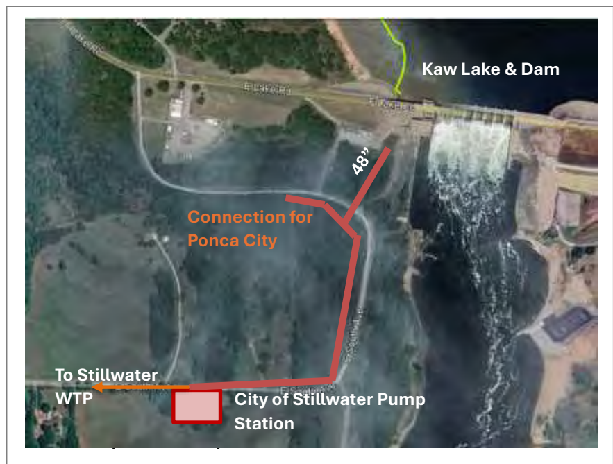
Figure 2-2 Kaw Lake Intake Pipe for Stillwater and Ponca City
