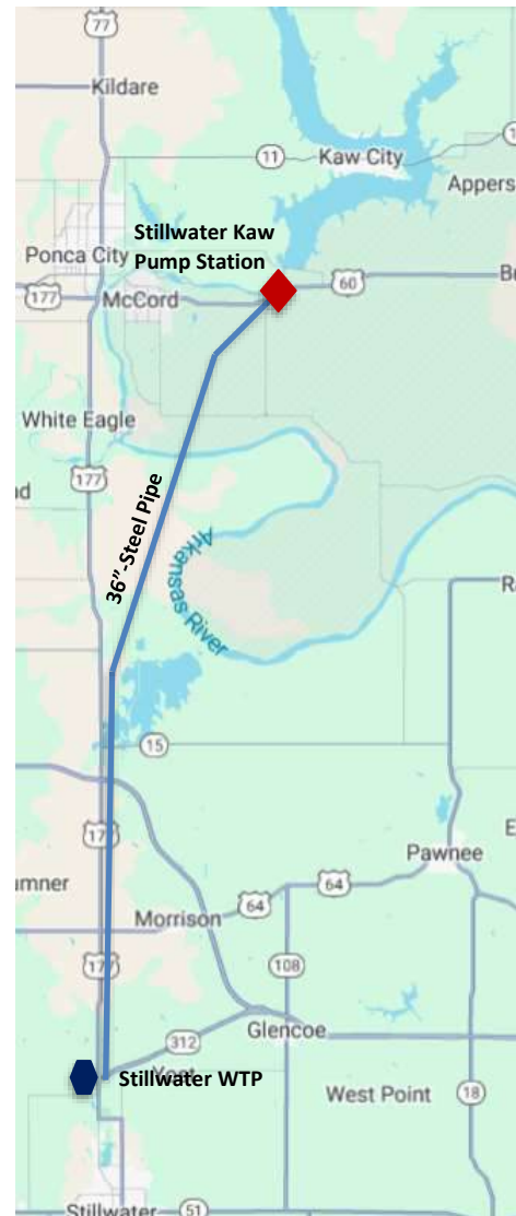
Figure 1-5 Stillwater Raw Water Conveyance System
